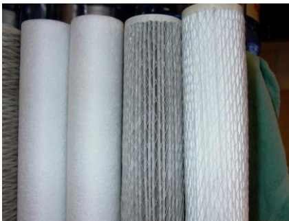
The second Poly Spun from the left was in the same amount of time as the NanoCeram filter, which is third from the left. The dirt that the NanoCeram filter caught went right through a five micron Poly Spun filter. The new and used Poly Spun filters look identical.
