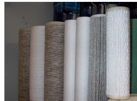
L to R: 1. Wound 20/5-micron filter (used 1-month); 2. New wound 20/5-micron filter; 3. Second wound 20/5 micron filter (used 1-month); 4. New Poly Spun 5-micron filter; 5. Third - Poly Spun 5-micron filter (used 1-month); 6. Fourth - NanoCeram filter (used 1-month); 7. New NanoCeram filter.
